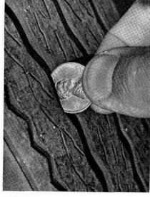
If your car is not equipped with tires incorporating the new "tread wear indicator" feature, now a federal standard, there is a simple method for determining when the tread is worn to the danger level: insert a penny with the head down into a center groove. If the top of Lincoln's head is visible, the tire is down to 1/16th of an inch depth, the minimum recommended for safety.
